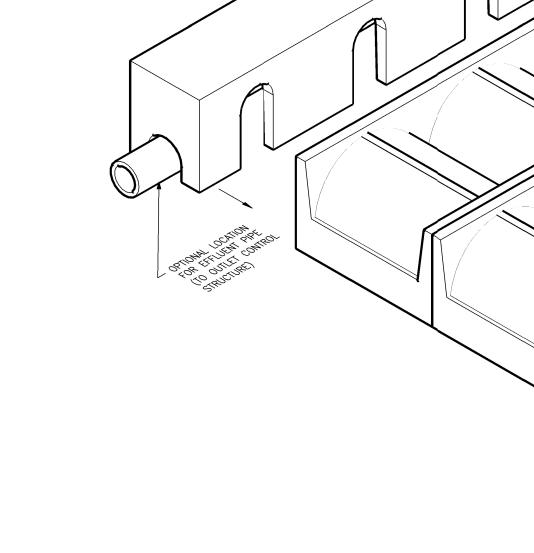
1. ACCESS OPENING(S) ARE TO BE LOCATED IN THE TOP OF MANIFOLD(S). OPENINGS MAY BE 24" DIA. FRAME/COVER AND/OR 24" x 45" FRAME/GRATE.
